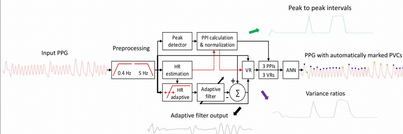
Figure 3: PPG based PVC detection and classification method scheme
