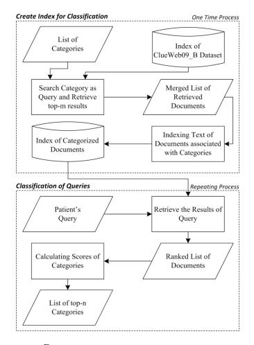
Fig. 1 The flowchart of the query classification process.
