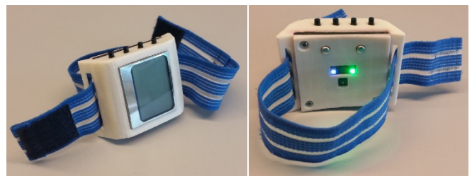
Fig. 1 Photos of the developed PPG wearable sensor: front (left) and back (right)
